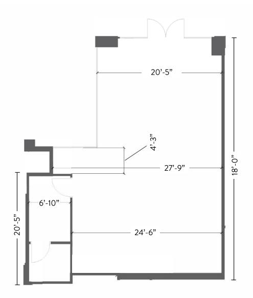
UNIT 201 **RETAIL AREA** 972 Square Feet **CEILING HEIGHT** 14' 5" POWER 225A, 120/208V **COOLING CAPACITY** 1,747 CFM **GENERAL EXHAUST** 13,000 CFM WATER 1" Line GAS No SEWER 4" Line GARBAGE Loading Dock LOADING Freight Elevator STORAGE Available Upon Request
