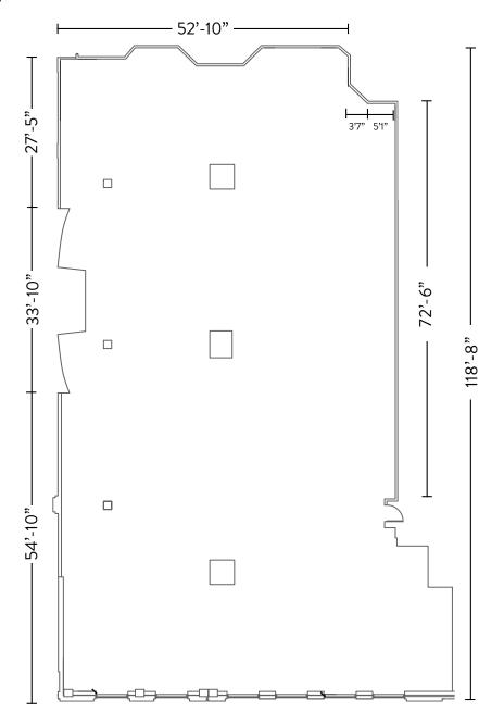
UNIT 360 **RETAIL AREA** 7,368 Square Feet **CEILING HEIGHT** 14'5" U/S of Slab POWER 120/208 V, 225A COOLING Two Units - 1000 & 1800 CFM WATER 3/4" Line GAS No SEWER 11/2" Line GARBAGE Loading Dock LOADING Freight Elevator
