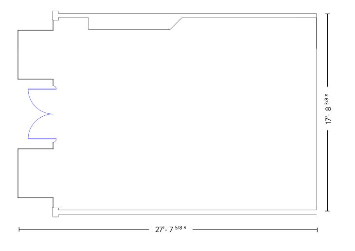
UNIT 334 **RETAIL AREA** 496 Square Feet **CEILING HEIGHT** 14'5" U/S of Slab POWER 100A, 120/208V COOLING 440 CFM **EXHAUST** 5,000 CFM WATER No GAS No SEWER No GARBAGE Loading Dock LOADING Freight Elevator
