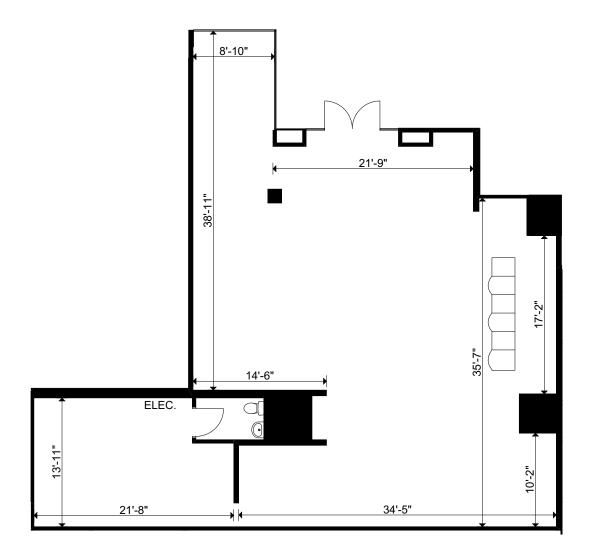
UNIT 205 **RETAIL AREA** 2,118 Square Feet **CEILING HEIGHT** 10' to Underside T-Bar POWER 60A, 120/208V HVAC Two Units - 4 & 10 Tons WATER 11/2" Line GAS No SEWER 3" Line GARBAGE Loading Dock LOADING Freight Elevator **STORAGE** Available Upon Request
