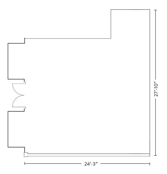
UNIT 338 **RETAIL AREA** 662 Square Feet **CEILING HEIGHT** 14' 5" POWER 225A, 120/208V **GENERAL EXHAUST** 2,000 CFM WATER 1/2" Line GAS No SEWER 4" Line GARBAGE Loading Dock LOADING Freight Elevator **STORAGE** Available Upon Request
