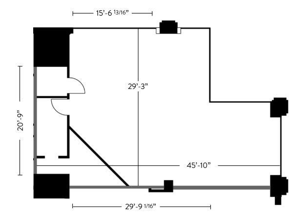
UNIT 145 **RETAIL AREA** 1,210 Square Feet **CEILING HEIGHT** 15' POWER 225A, 120/208V **GENERAL EXHAUST** 13,000 CFM WATER No SEWER 2" line GAS No GARBAGE Loading Dock LOADING Freight Elevator
