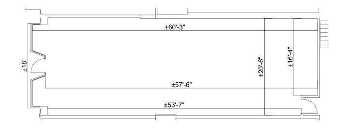
UNIT 340 **RETAIL AREA** 1,259 Square Feet **CEILING HEIGHT** 14'5" U/S of Slab POWER 225A, 120/208V **EXHAUST** 5,000 CFM **HVAC** 1 Ton per 300 sq ft WATER 3/4" Line GAS No SEWER 4" Line GARBAGE Loading Dock LOADING Freight Elevator
